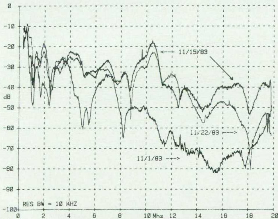
Fig. 3. Variation in attenuation on different days (resolution bandwidth = 10 kHz).
